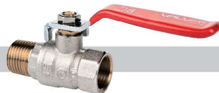
ONYX Full-port ball valve with nut on stem and steel lever (female-male version)
